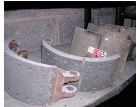
Figure 41 Asbestos brake linings for quarry vehicles
