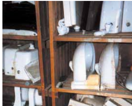
Figure 40 Asbestos-reinforced toilet cistern
