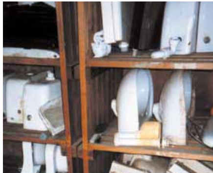
Figure 40 Asbestos-reinforced toilet cistern
